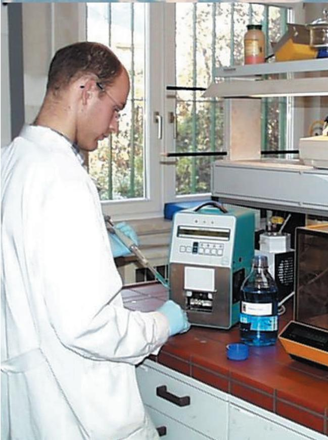
GRABNER INSTRUMENTS GmbH is one of the few manufacturers which produce instruments which are suitable for both on-site and laboratory operation. The Austrian armed forces uses Grabner instruments to determine the flash point [i], flow properties of lubrication grease [ii] according to KESTERNICH and measure the vapour pressure [iii].
