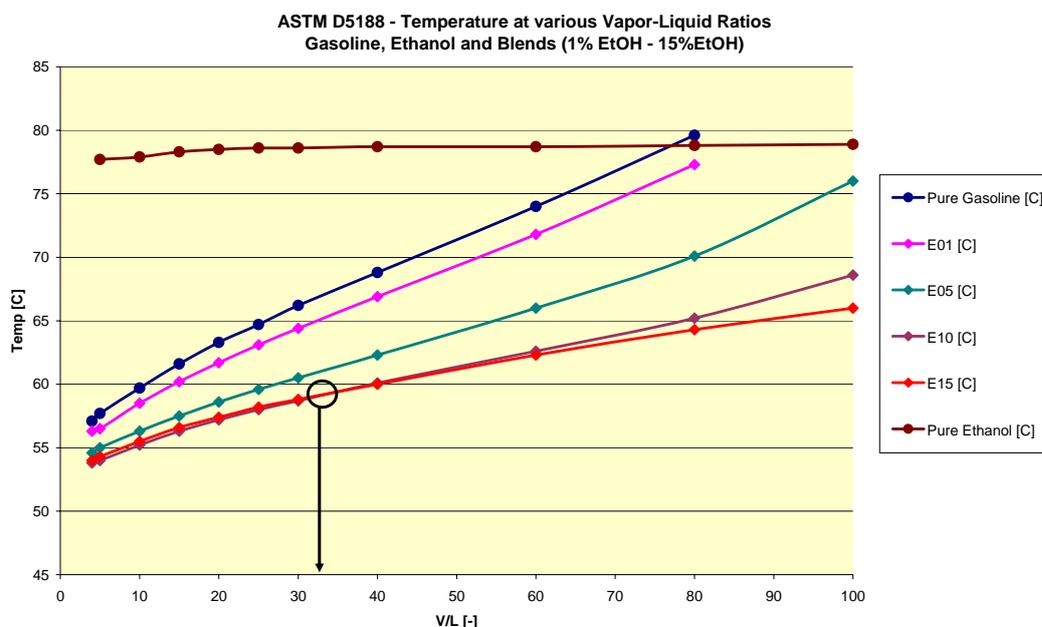
Fig 1: Temperature changes at various V/L ratio for 1%, 5%, 10% and 15% Gasoline-Ethanol blends.
